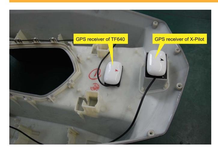
3) Fix the TF640 and X-Pilot as usual, including transmitter, transducer, Antenna, etc
