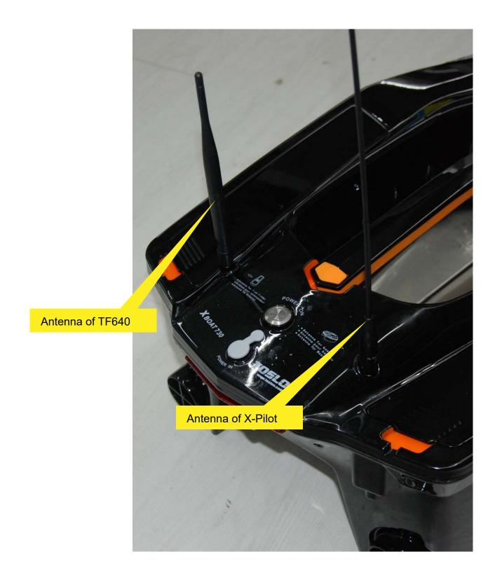
4) Use cable-1 and cable-2 to power transmitter of TF640 and X-Pilot
