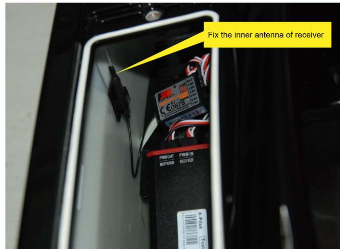
2) Fix the GPS receiver for TF640 and X-Pilot. To do this, you need open the housing of Xboat730 bait boat as following.
